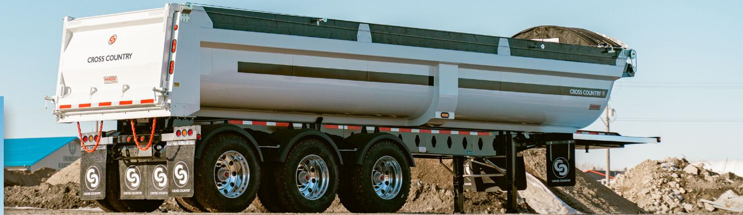
**Cross Country Manufacturing's Full Frame End Dump trailers are engineered with a drop frame design and lower tipping hinge to provide increased stability while unloading.**
